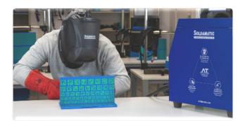
Soldamatic Robotics is a robotic welding solution to train the operators, as well as to evaluate the programming of complex welding before its production in real-time.
